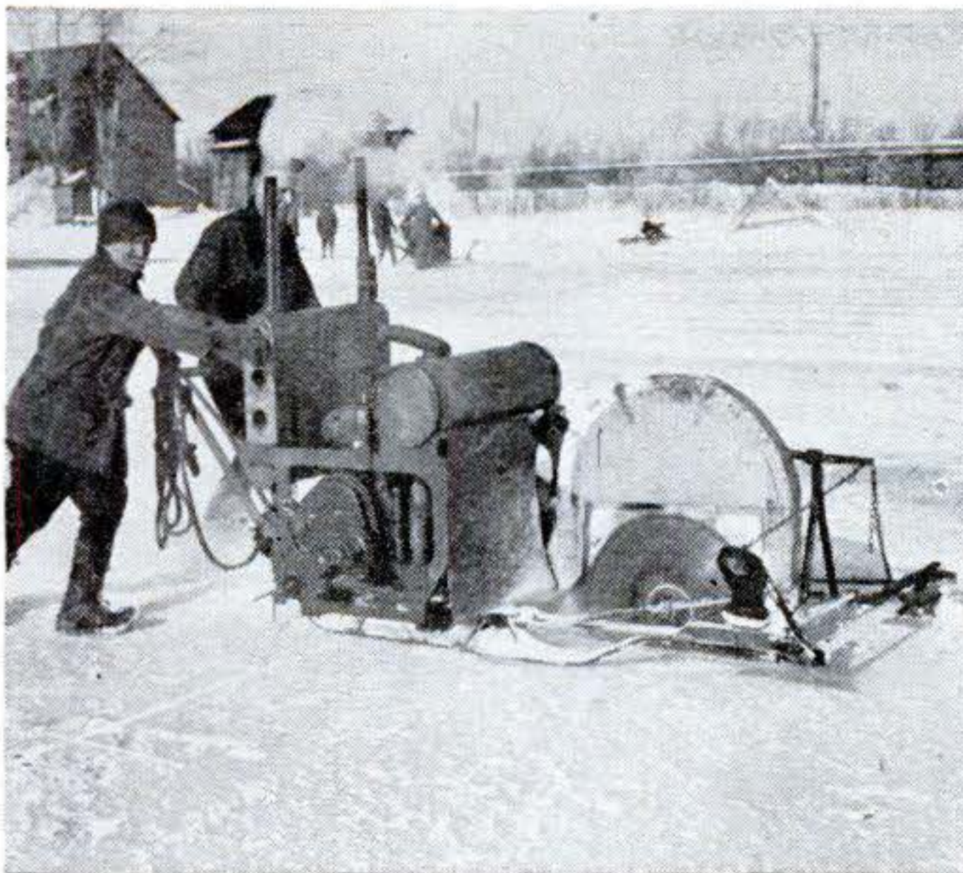
4. Gasoline-powered saws take over. Working in teams of two, one laterally and the other longitudinally, they cut cakes measuring 32 by 22 inches. Blades bite 10 inches into the ice.
